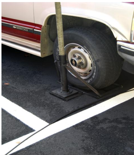
Drive-on mount for erecting an antenna on a push-up pole
